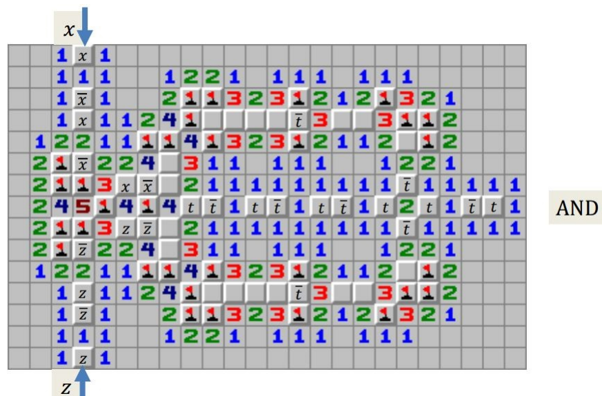
Figure 3.10: AND gate for Minesweeper.
